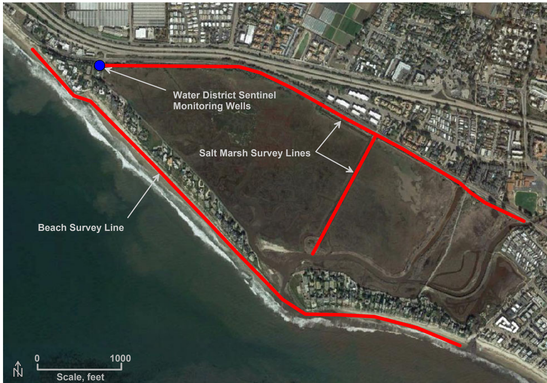
Figure 1. Proposed Geophysical Survey Lines Carpinteria Groundwater Basin Groundwater Sustainability Plan
